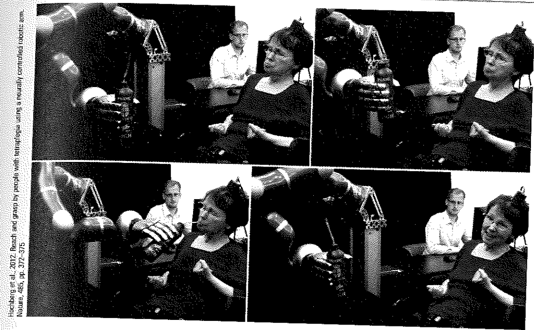
Figure 12.3 Mind over matter. A series of strokes left Cathy paralyzed for 15 years, unable to make even simple arm movements. Now, thanks to a tiny, 96-electrode implant in her brain's motor cortex, she is learning to direct a robotic arm with her thoughts (Hochberg et al., 2012).
